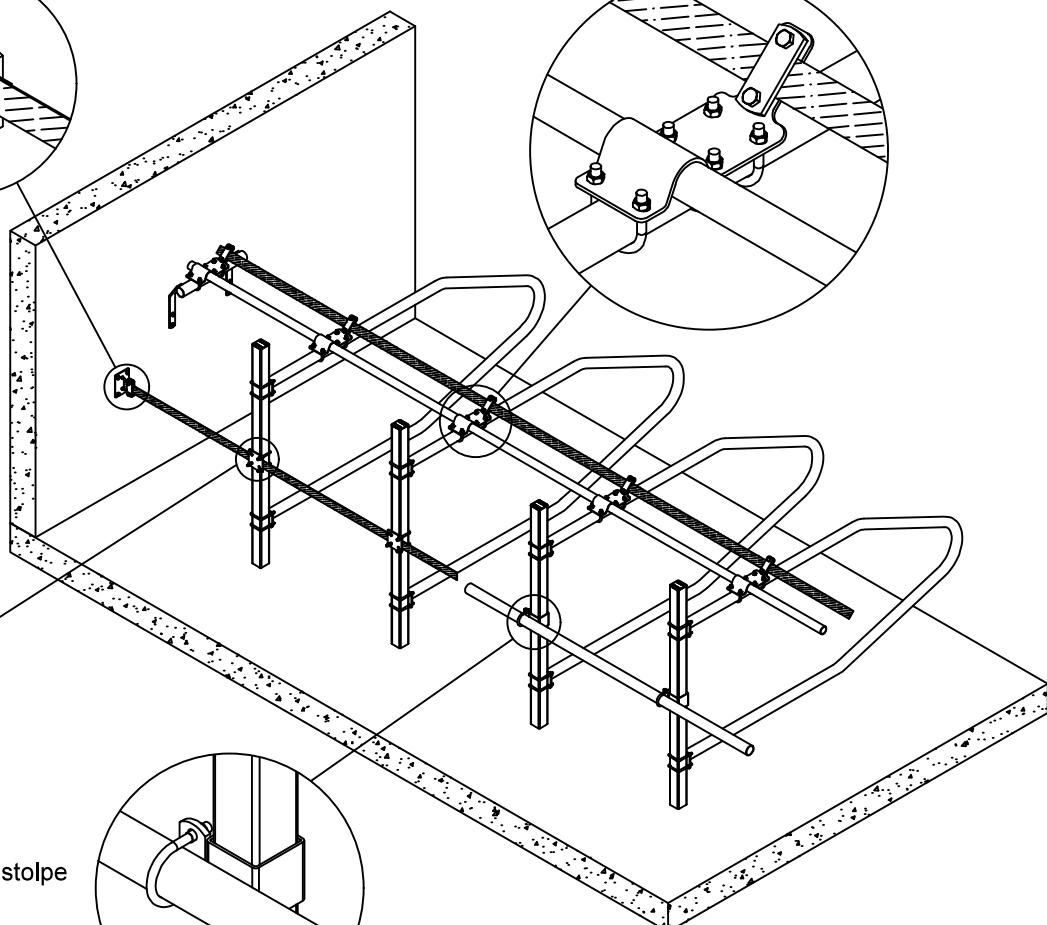
**Fig. 1** Monteres med: M10x80 Eksp. bolt
